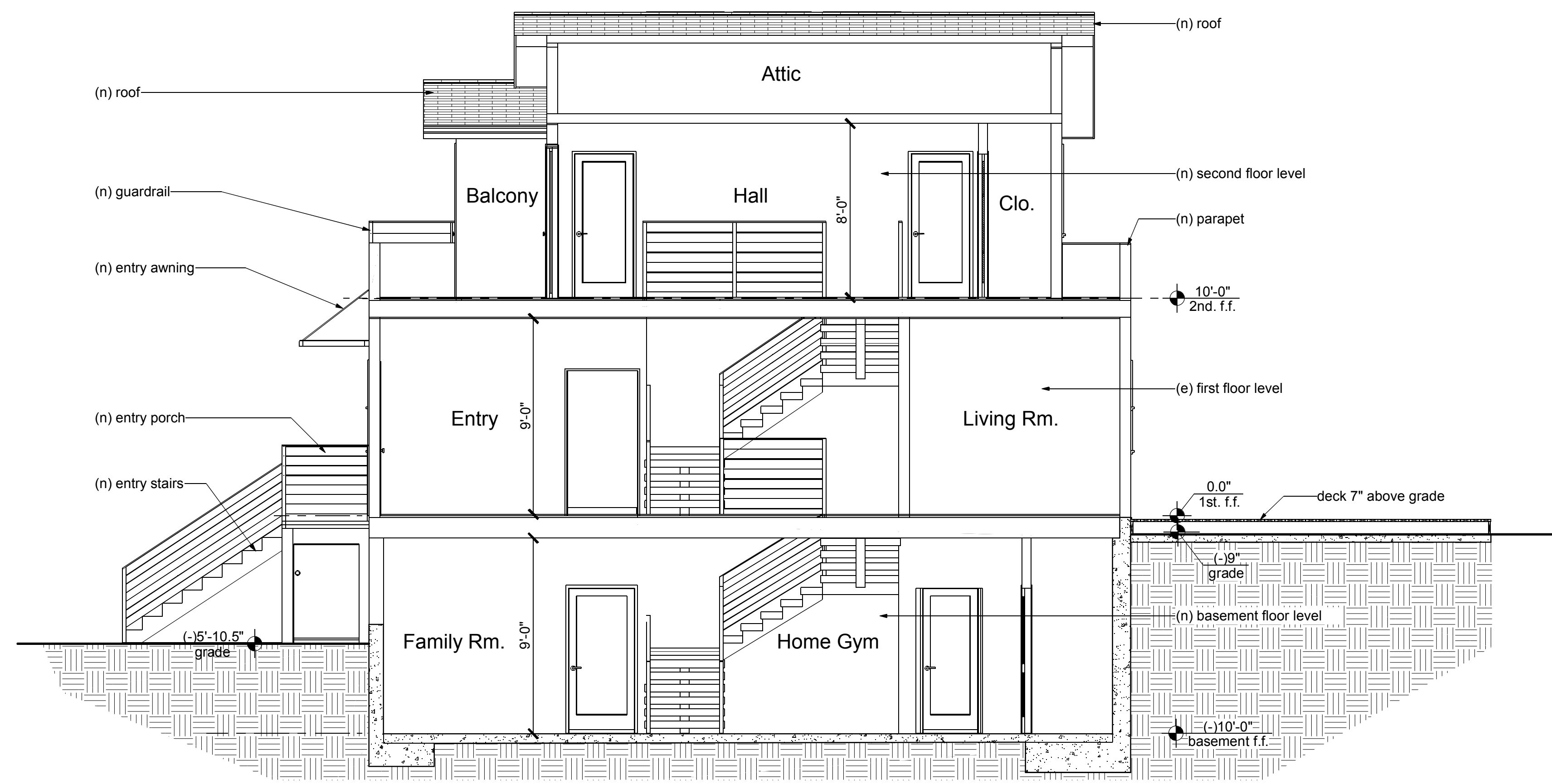
1 Proposed Building Section
